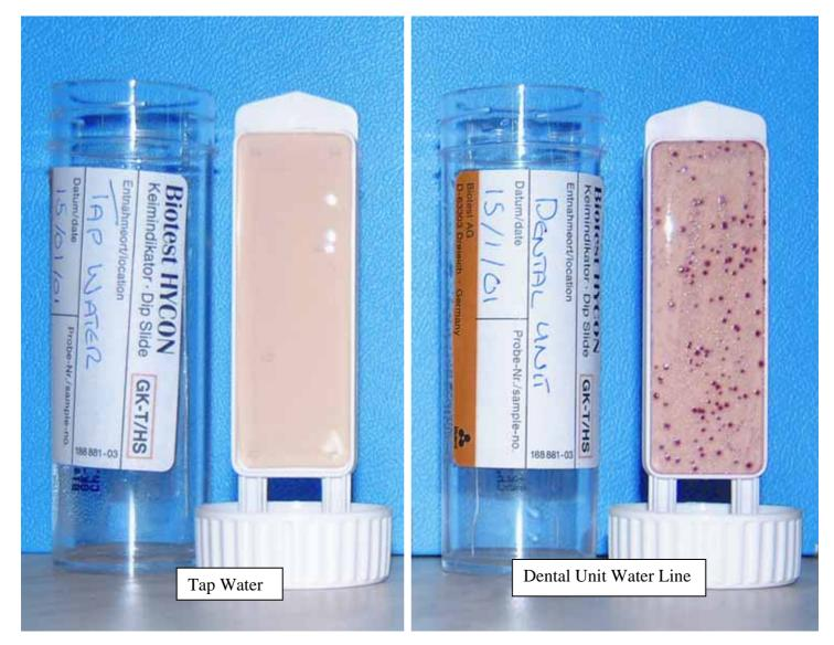
The Dip Slides illustrate above show the difference between Tap Water and the untreated water within most dental water lines. The Dental Unit clearly does NOT conform to the current E.U guidelines. By using our system, we can produce drinking quality water from your Dental Unit such that results post-treatment will be as per the Tap Water, above. The system is easy to use and will maintain potable water from your unit.
